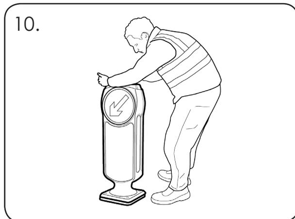
10. To test that the Bollard is working. Cover the solar panel and Light Dependent Resistor [top of the Bollard] for approximately 10 seconds. The sign face should illuminate.
